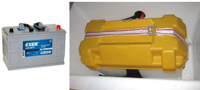
Engine battery: 2 x 120A
