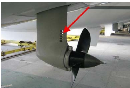
Seawater intake Intake filter
