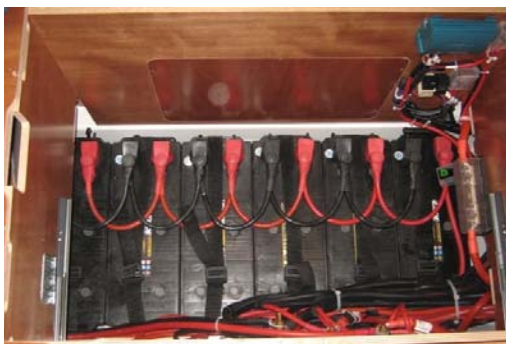
Service batteries: 6 x 120A
